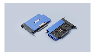
A PCIe card containing the IBM AIU. (Credit: IBM.)
